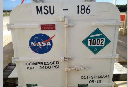
DOT-4 tube skid
